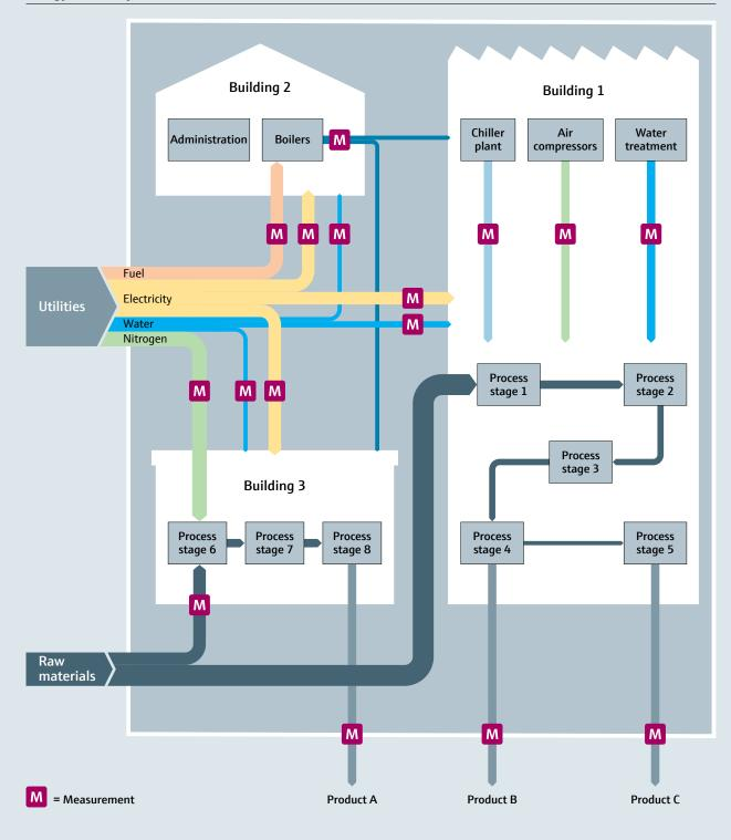
Procedure for measuring material and energy flows as the basis for sustainable energy management
