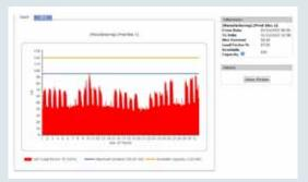
Track consumption profiles of a measuring point over various days of the week
