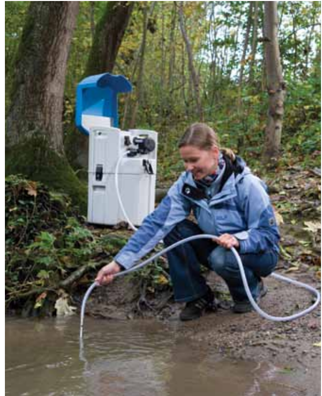
Quick and easy: Direct sampling on the banks of a stream with the mobile Liquiport CSP44
